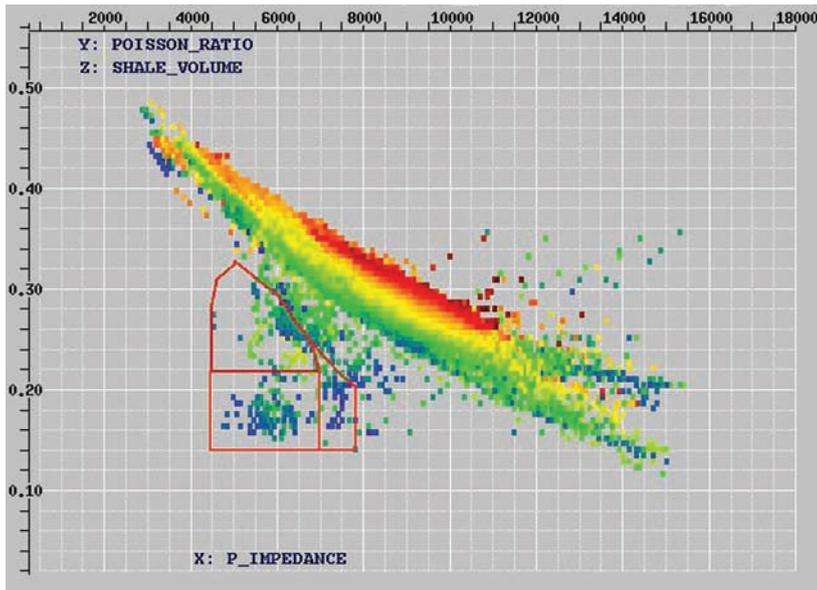
**Fig 2.** Crossplot of well data isolates the zone of sands using the attributes of P impedance and Poisson's Ratio. Once defined, such criteria can be applied to the seismic-generated P impedance and Poisson's ratio to predict rock property spatial distribution
