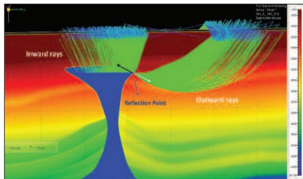
The local angle domain separates inward and outward rays from a common image point (BP TTI model). (Image courtesy of Paradigm)
