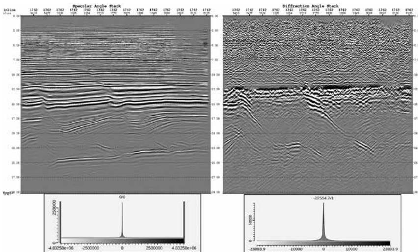
**Figure 1** Specular reflection stack (left) and diffraction stack (right) with their respective value ranges (data courtesy of Seitel).
