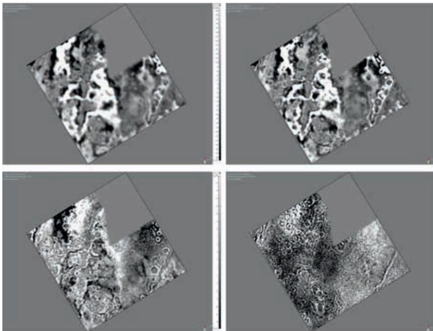
**Figure 4** Depth slice 1372 m, different ranges of dip were stacked. As we separate reflections from diffraction energy, karsts and faults are revealed with higher resolution. From upper left to lower right: all dips stacked (0°-45°), 0°-15°, 15°-30°, 30°-45°.
