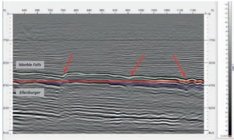
**Figure 3** Specular reflection stack with interpreted seismic events (Marble Falls and Ellenburger). The red horizontal line at 1372 m is the reference for further analysis.
