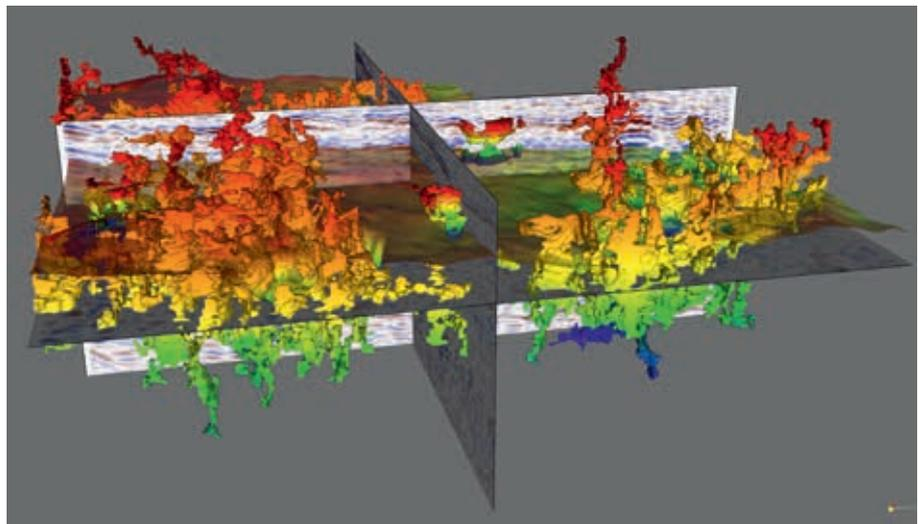
**Figure 6** Detected complex geobodies (from curvature attribute generated from 15°-30° partial dip stacking) corresponding to karst features, jointly visualized with diffracted stack attribute and top of the Ellenburger formation (semi-transparency).
