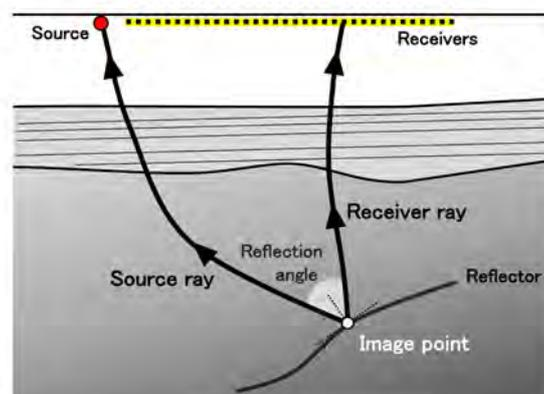
**Figure 1** Schematics of the common reflection angle migration method. The local reflection angle is defined based on the source ray and receiver ray from subsurface imaging point to surface sources and receivers.
