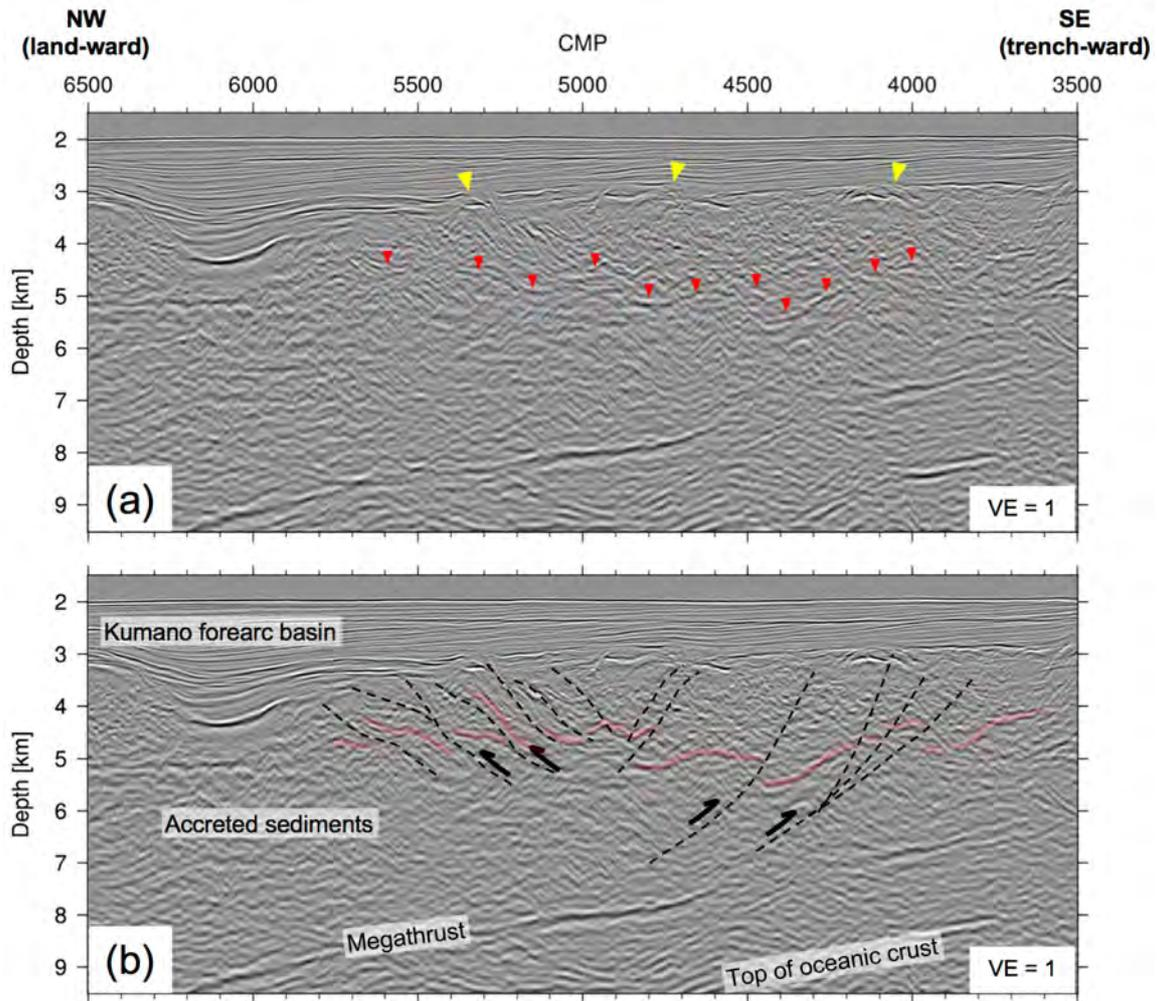
**Figure 3** (a) Final common reflection angle migrated section of the target area indicated in Figure 2b. Yellow triangles indicate folded structures just below the forearc basin, and red triangles indicate reflectors in the accreted sediments. (b) The same section as (a) with interpretation of multiple thrust faults (black dashed lines).
