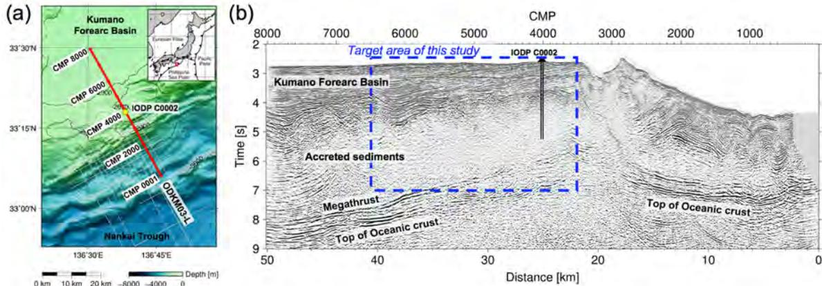
**Figure 2** (a) Map of the 2D seismic survey in the Nankai Trough off the Kii Peninsula, southwest Japan. The red line is the processed line, ODKM03-L, and the yellow circle indicates the scientific ocean drilling hole IODP C0002. (b) The legacy section obtained by pre-stack time migration in 2004. Our target area is indicated with the blue dashed line box.
