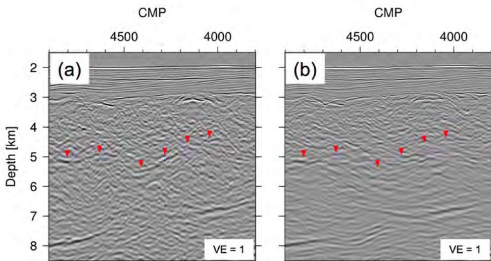
**Figure 4** Comparison of migration results by (a) common reflection angle migration, and (b) conventional Kirchhoff migration using the same pre-processed data and velocity model.
