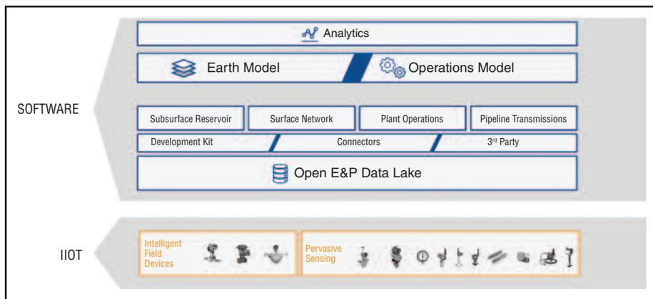
Figure 2 shows a data lake between the IIOT sensor data and subsurface model data. This new IT approach is providing the foundational layer for creating a single, interconnected digital twin for unified analytics of the entire exploration, drilling, completion and production workflow, rather than piecemeal efforts.
