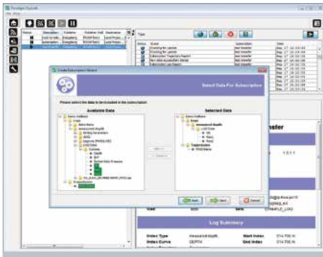
▲ Setting up an OpsLink subscription to transfer WITSML log data to a Paradigm Epos database
