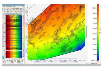
▲ Full-azimuth common reflection point gather from an Eagle Ford Shale dataset recovering 1% anisotropy at a depth of 11,800 ft. Fracture and stress intensity and orientation map from full-azimuth residual moveout inversion. Data courtesy of Seitel.
