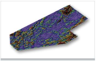
Co-visualization of fracture/stress intensity from full azimuth inversion and fracture imaging from the Coherence Cube attribute. Data courtesy of Seitel.
