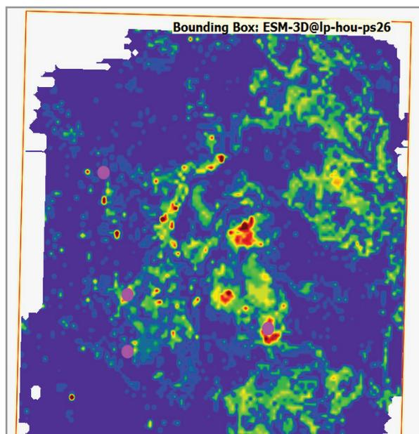
Figure 4 – Oil-filled packstone two-way time thickness map
