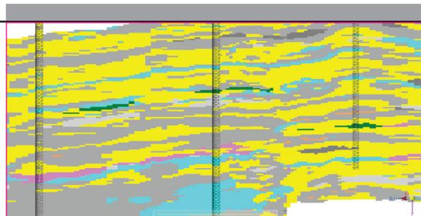
Figure 2 – An excellent tie between the facies logs at the three wells and the 3D seismic facies classification results. The common color scheme in Figure 1 is used, the pay is dark green Facies 5, oilfilled packstone.
