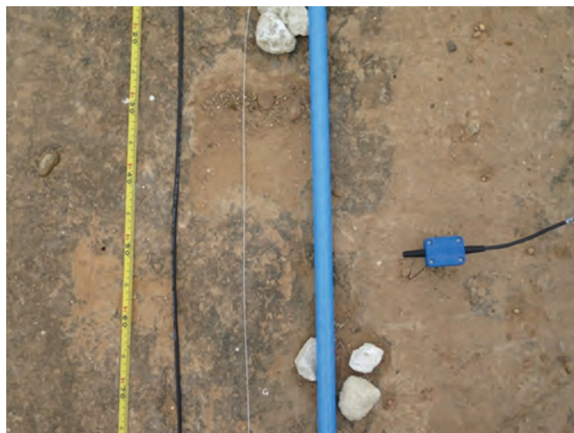
Figure 1. The four coincident 2D seismic lines in the experiment. The geophone line consisted of 96, 14 Hz geophones at 1.5 m spacing. The blue cable is the helically wrapped cable, referred to as cable 1. The thin white one is a nearly bare single-strand fiber (cable 2). Cable 3 (black) is an armored single-strand fiber. The image shows approximately 80 cm of the three cables (the tape measure in yellow).
