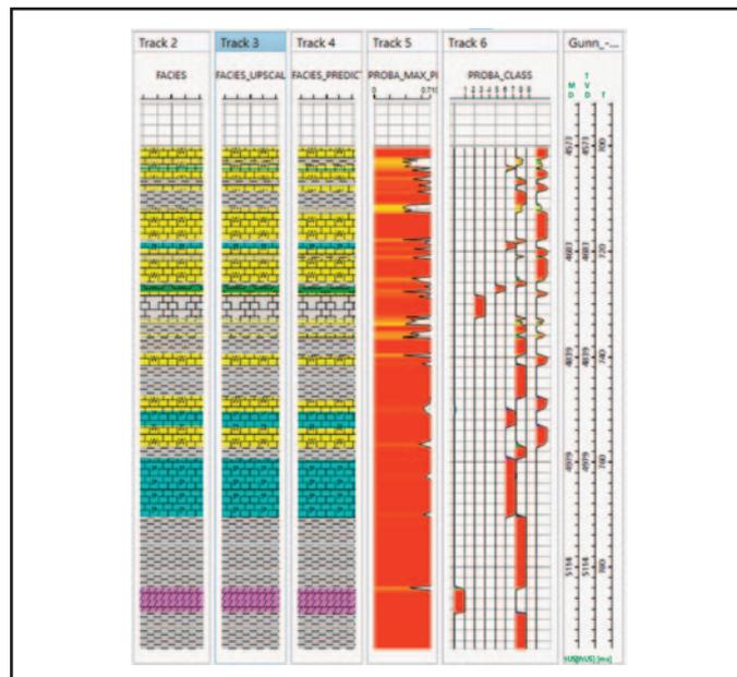
run simultaneously to predict facies and avoid biasing any of the neural network architectures. To train the neural networks, facies at the well and seismic data extracted along the wellbore in the interval of interest are used as input data (the hard training dataset). A major benefit of this technology is its ability to combine the full dimensionality of the prestack data, which carries more information, with any type of seismic attributes.
