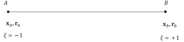
Figure 3 Scheme of two-node Hermite element.
