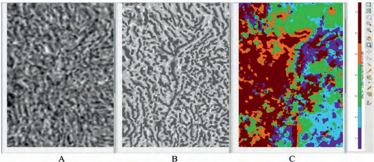
**Figure 8** Interpretation of two maps showing fault/fracture systems and a seismic facies map: (A) Fault map obtained with the diffraction filter technology from directional gathers. (B) Fault map obtained from diffraction cube through machine learning using the principal component method. (C) A map of seismic facies in the azimuthal sector along the HTI axis of symmetry.
