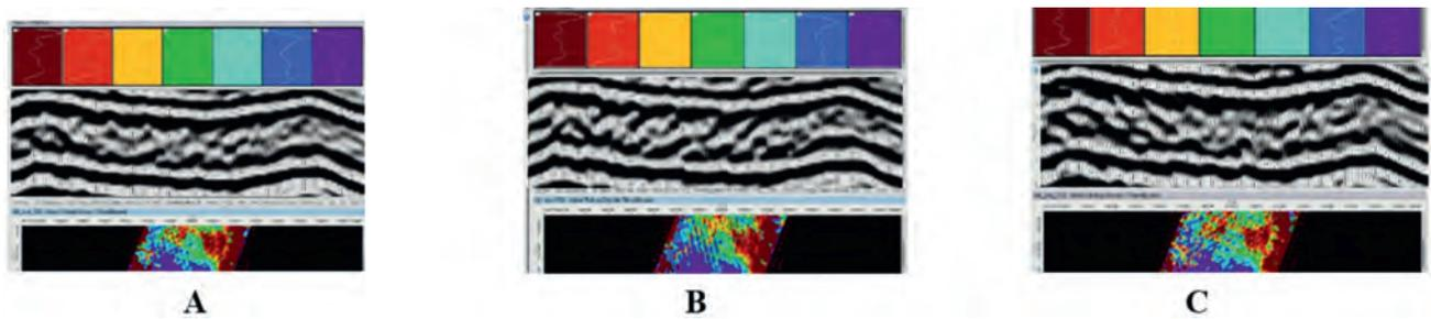
**Figure 2** Changing the shape of the traces and the classes depending on azimuth. Lower Chalk (K1), Neokom, Western Siberia. (A) Full Azimuth 0-360°, (B) Sector 135°-180°, (C) Sector 45°-90°.
