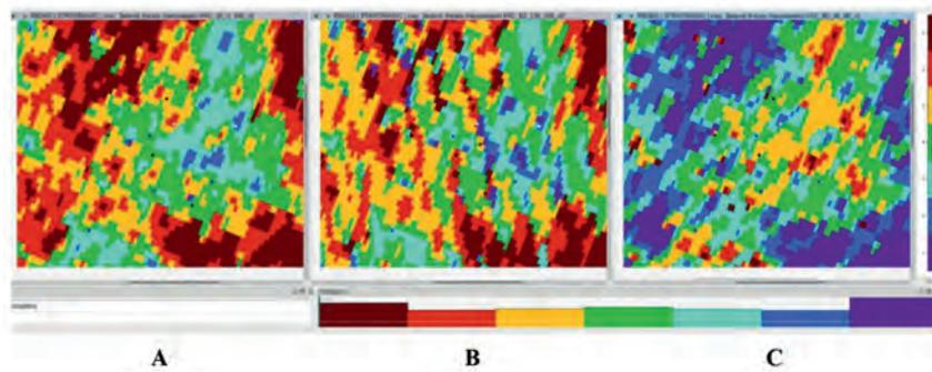
**Figure 3** Maps of seismic facies in the interval of oil-saturated reservoirs for different azimuth sectors: (A) Full azimuth 0-360°, (B) 135°-180°, (C) 45°-90°. Pinch-out zones, Lower Cretaceous (K1), Neokom, Western Siberia.
