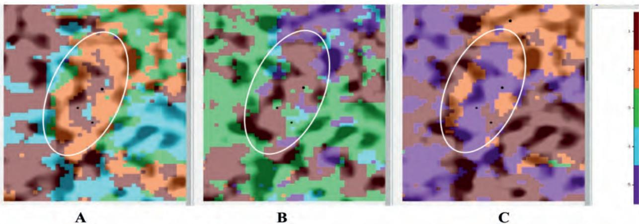
Figure 5 Distribution of seismic facies in a carbonate reservoir depending on the azimuthal direction of the stack sectors. (A) along the HTI axis of symmetry, (B) across the HTI axis of symmetry, (C) full-azimuthal stack.
