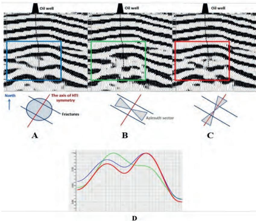
**Figure 1** Changes in the trace shape depending on the azimuth direction of the seismic sector analysis in the oil-saturated reservoir interval. (A) full azimuth stack: 0-360°; (B) azimuthal sector stack: 115-145°; (C) azimuthal sector stack: 25-55°. Paleozoic basement / West Siberia. (D) – Amplitude-frequency spectra of the three images. Paleozoic basement in West Siberia.
