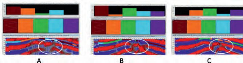
**Figure 4** Selection of templates (classes) for sectorized azimuth analysis of seismic facies: (A) = 60°-90°, (B) = 140°-170°, (C) = 0°-360°. Below are the stacks for the different azimuthal sectors. The zones of the oil-bearing part of the reservoir are marked with ovals.
