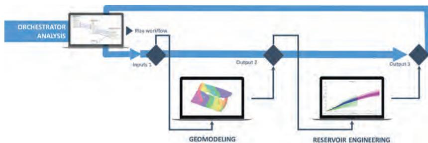
**Figure 3** AspenTech automated and integrated subsurface workflow principle. The modelling tasks are played automatically in sequence. The workflow, inputs and outputs are controlled by the workflow orchestrator.
