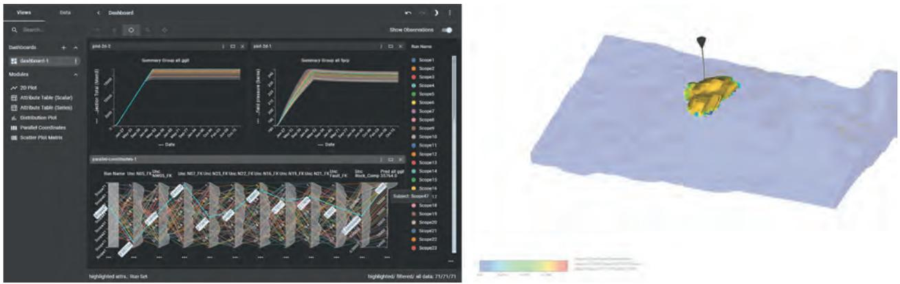
**Figure 6** Left: Interactive dashboard to post-process the ensemble of models generated. Total CO<sub>2</sub> injected, field pressure, and range and values of uncertainties are displayed in the dashboard. Right: 3D view of the dynamic model corresponding to the highlighted simulation (blue) on the left.
