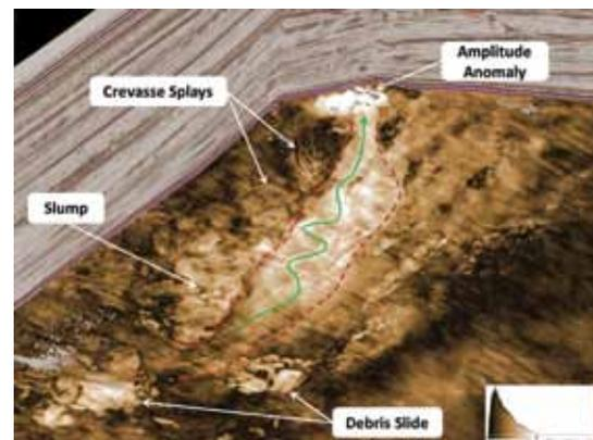
**A stratigraphic slice through a deepwater depositional interval reveals slump features, debris slides, and an interpreted fluid migration fairway leading updip (green arrow) to a high-amplitude anomaly associated with a structural high (potential direct hydrocarbon indicator). (Data courtesy of AWE Ltd.)**
