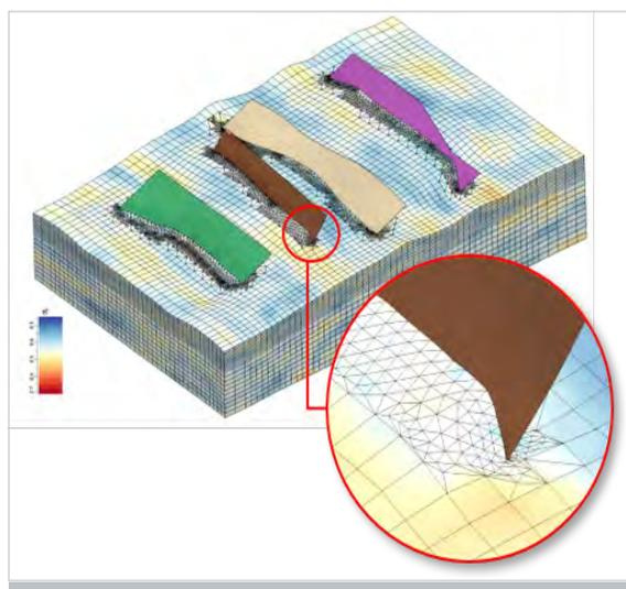
▲ 3D mechanical hybrid grid including hexahedral and tetrahedral elements to perfectly capture faults and fine-scale heterogeneities impacting the storage complex geomechanical behavior.
