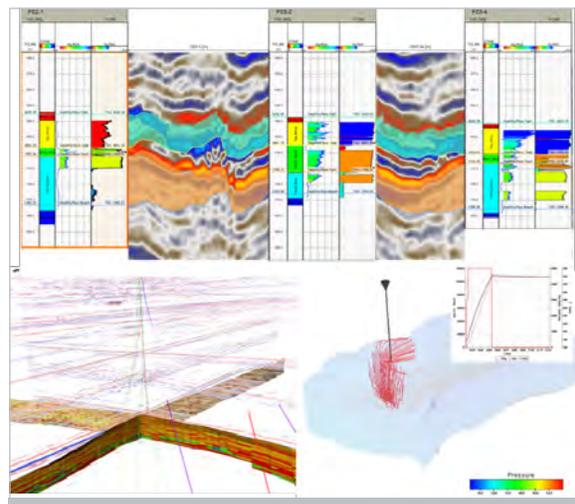
▲ Static and dynamic modeling to support the evaluation of storage capacity.
