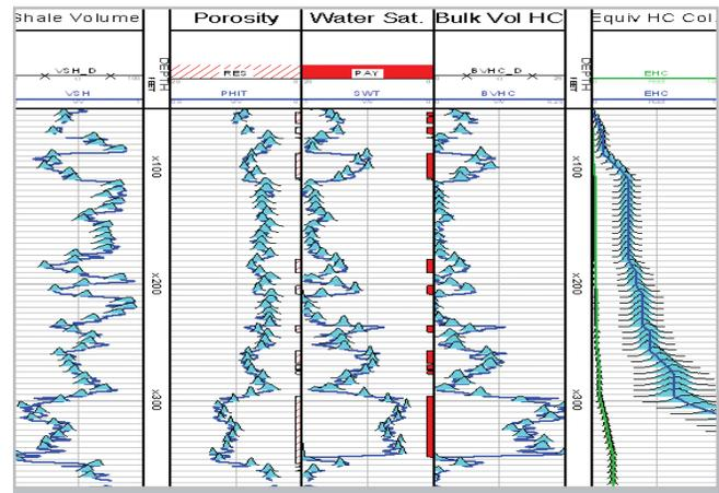
▲ Output log showing distributions for each main petrophysics output on a frame-by-frame basis
