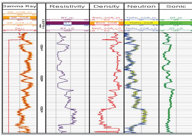
▲ Input logs after environmental corrections with the base case, low and high case scenario
