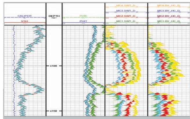
▲ Log plot showing the results of water saturation and bulk volume hydrocarbon from different saturation models
