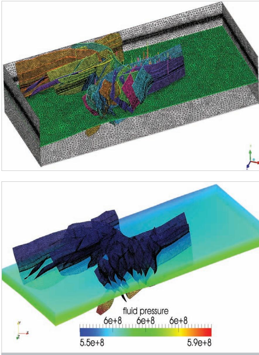
▲ Figure 2: Reservoir grid, with tetrahedral mesh for honoring the complex fault structure, with a discrete well representation (left), and with pressure initialization in the main reservoir unit and along fault planes (right)
