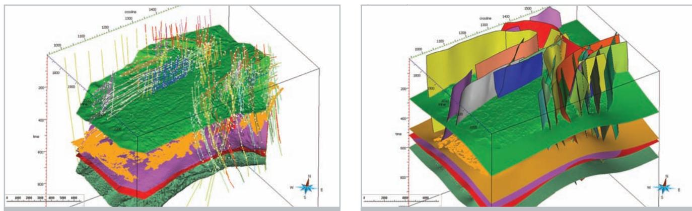
▲ Figure. 1: In two-way-time domain: fault interpretation as fault sticks and main stratigraphic horizons (left), from basement (dark green) to ground level (top); water-tight structural model (right), honoring the complex fault system and the stratigraphic unconformity (onlapping deltaic sand series) between red and purple horizons. (View set-up: vertical exaggeration x2)
