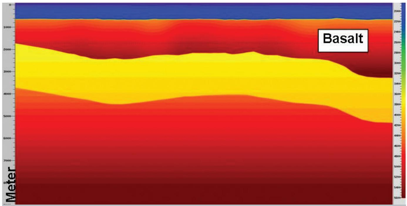
▲ Interval velocity model used for the synthetic full-wave elastic.
